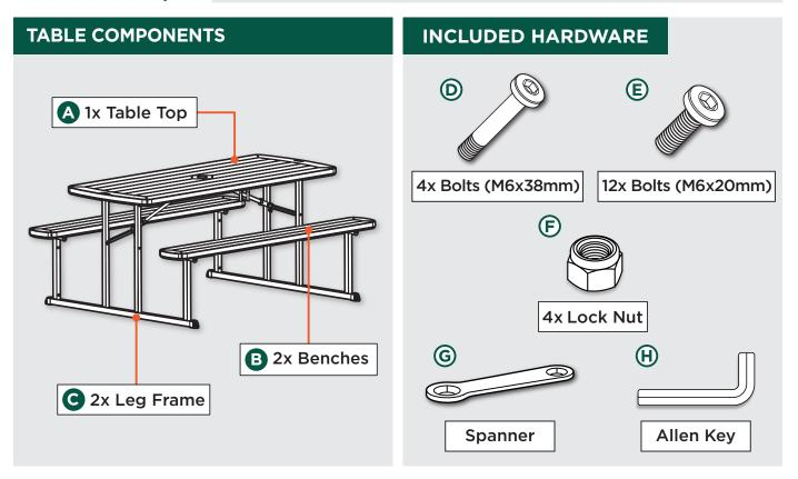
Place Table Top A upside down on a clean, dry, soft surface. Use Bolts E, Long Bolts D and Nuts F to attach Leg Frame C to Table Top, and lock into place. Turn Picnic Table upright after completed this step.
