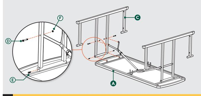
Ensure that all bolts are fastened tightly.
