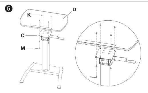
With the pencil tray facing the same direction as the pneumatic lever, attach the Desktop ( $\mathbf{D}$ ) onto the top of the Adjustable Fitting ( $\mathbf{C}$ ). Using screws ( $\mathbf{K}$ ) tighten with Hex Key ( $\mathbf{M}$ ).
