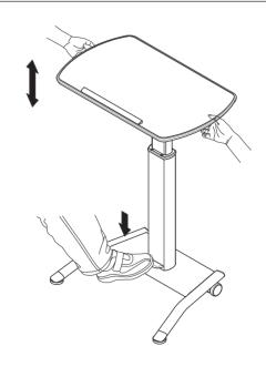
To adjust the Desktop (**C**) height, grab the Desktop with both hands while stepping on the pneumatice lever of the Base (**B**) to raise or lower the Desktop.
