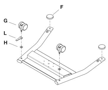
Attatch the Adjustable Pads (**F**) to the Outter Plugs turning them until tight. Using the Spanner (**L**) and washer (**H**), attach and tighten the Casters (**G**).
