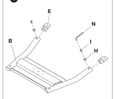
Turn the Base (**B**) over to the underside, slide the Outter Plugs (**E**) onto the Base and align the screw holes. Using the 5mm Hex Key (**N**) insert screw (**I**) and washer (**H**) and tighten the Outter Plugs to each side.
