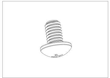
Serrated Screw Quantity: 8 (12 on Centric, 84" and 96" Wide)
