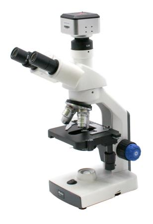
This microscope features a Siedentopf trinocular head, low-drive mechanical stage, spring specimen holder, easy to use coaxial focusing system, 0.5X C-mount and 1.25 condenser. M2652CT-3 is also rechargeable, with cool and efficient dimmable LED illumination.
