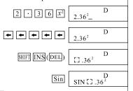
When SHIFI INS are pressed, the space that is opened is displayed as ." []". The function or value assigned to the next key you press will be inserted in the []. To exit from the insertion mode, move the cursors, or press SHIFI INS, or press =.
