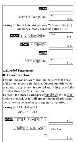
Numeric values with 12 digits for a mantissa and 2 digits for an exponent can be stored in the Ans memory. The Ans memory is not erased even if the power of the unit is turned OFF. Each time [=], Shift [%], M+, Shift [M-], and STO oc=A~F,M,X,Y) is pressed, the value in the Ans memory is replaced with the new value produced by the calculation execution. When execution of a calculation results in an error, however, the Ans memory retains its current value.
